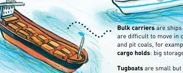
**Bulk carriers** are ships that transport goods that are difficult to move in containers. Ores, grains, and pit coals, for example, are transported in **cargo holds**: big storage tanks on board.
