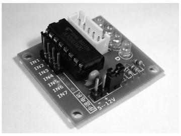
*Illustration 73: The stepper motor driver module*
