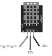
Illustration 50: The DHT11 measures Temperature and Humidity
