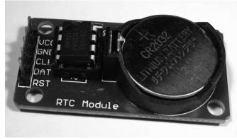
Illustration 90: The RTC module with 3 V coin cell
