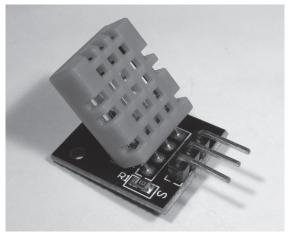
Illustration 49: DHT11Temperature/Humidity sensor
