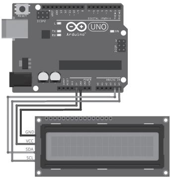
Illustration 31: I2C LCD with the Arduino
