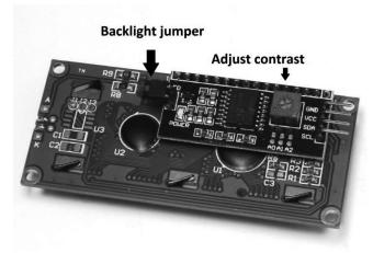
Illustration 30: The LCD module from the back
