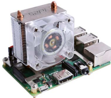
Figure 1.3 Raspberry Pi 4 CPU fan ( www.seeedstudio.com )
