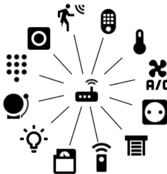
Figure 1.1 A home automation system consists of a central gateway and various controllable devices and sensors.
