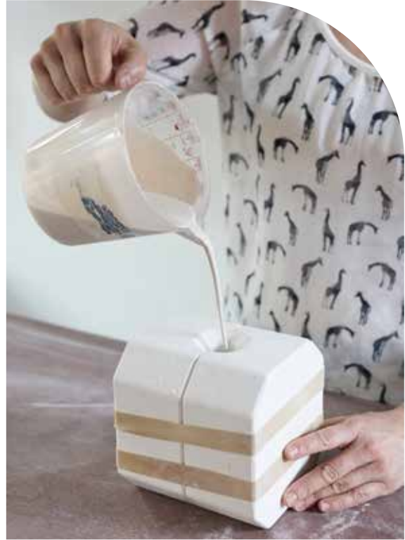
Liquid porcelain being poured into a plaster mould. After pouring, a thin layer of porcelain remains in the mould. When dry, the mould can be carefully removed and the piece can then be finished as desired.
