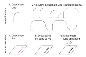
1. Draw main Line using specific dimensions. The Line can have any geometry, from a straight line to a curve.
