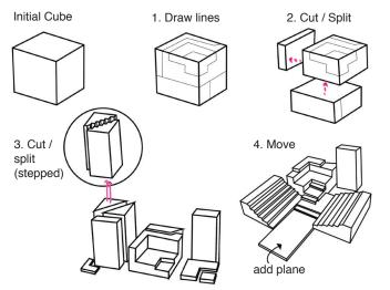
1. Draw lines on the cube. The lines can be rectanglular or have any geometry, such as curves.
