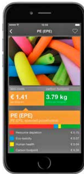
With the Idemat Light app you can make a simple LCA calculation according to the Fast Track method, using the data and the selection method. You can open an LCA, and add materials and processes to it with the required quantities. You can even calculate the eco-costs of products with an Environmental Declaration. (idematapp.com)
