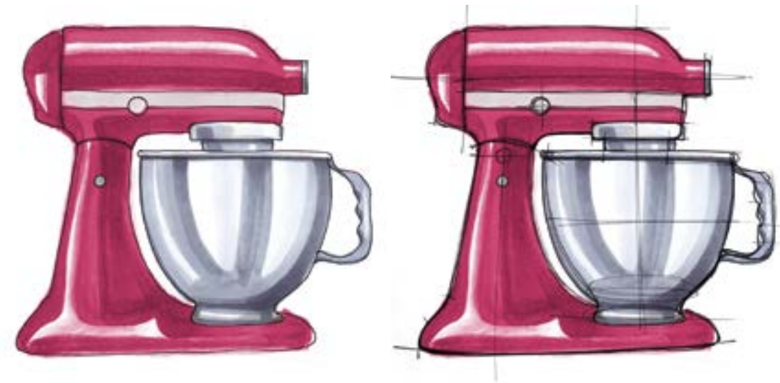
1) With single lines, the drawing looks like part of a comic strip. 2) With 'sketch' lines, the drawing looks more like an intelligent design.
