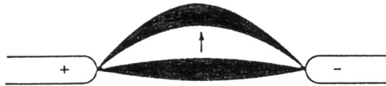
Figure 1.3. Formation of the arc shape in the case of rod-shaped electrodes, placed horizontally at large distance.
