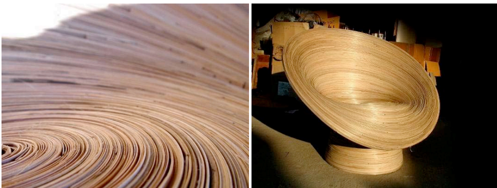
Figure 1.9: Coiling is a non industrial processing technique that can create surprising effects; chair design (right) by Jared Huke
