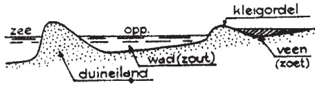
Figure 1 Sketch of the 4 alluvial [A3] zones: dunes, wadden, silt, peat (fresh water) [A4].
