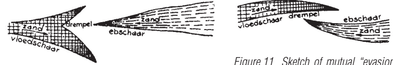
Drempel = delta ebschaar in delta vloedschaar Figure 10 Sketch of the mutual "evasion" of flood and ebb channels by means of a forked tongue [A21].
