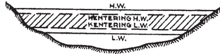
Figure 6 The lines of slack water are generally at a distance of 0.9 x tidal amplitude; in deep, wide estuaries less, in seas the distance is zero.
