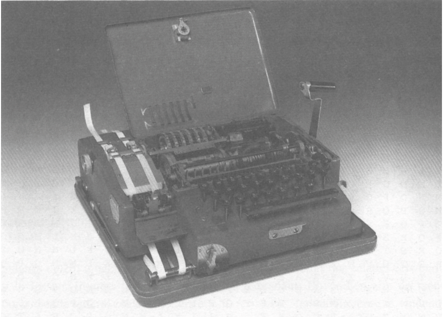
Figure 2.3. The Hagelin machine. The lower photograph clearly shows the coding wheels (1) and drum (2) (photographs by Facilitair Bedrijf TU Delft, Photographic Service).
