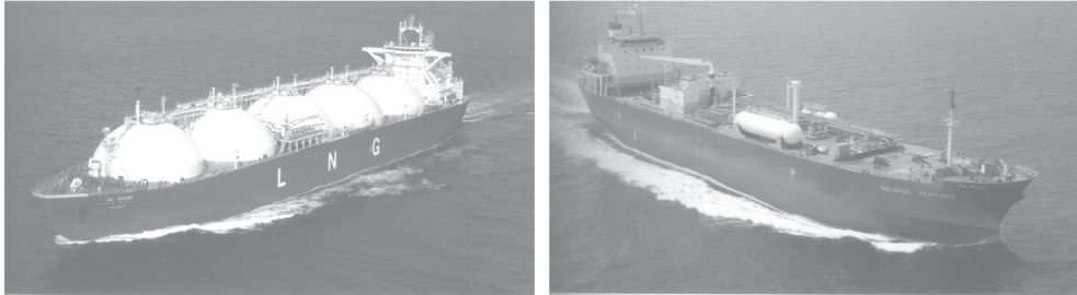
Figure 2.28 Examples of LNG-tankers (left) and LPG-tankers
