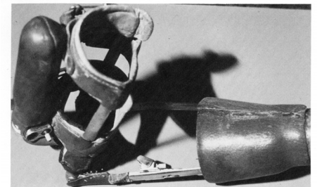
Figure 1.15 An early example of a pneumatically powered hand prosthesis. The supply pressure is presented at the gas duct #1 and displaces the pistons #2. These pistons drive the proximal phalanxes of the fingers. A mechanical coupling drives the distal phalanxes to the proximal phalanxes.
