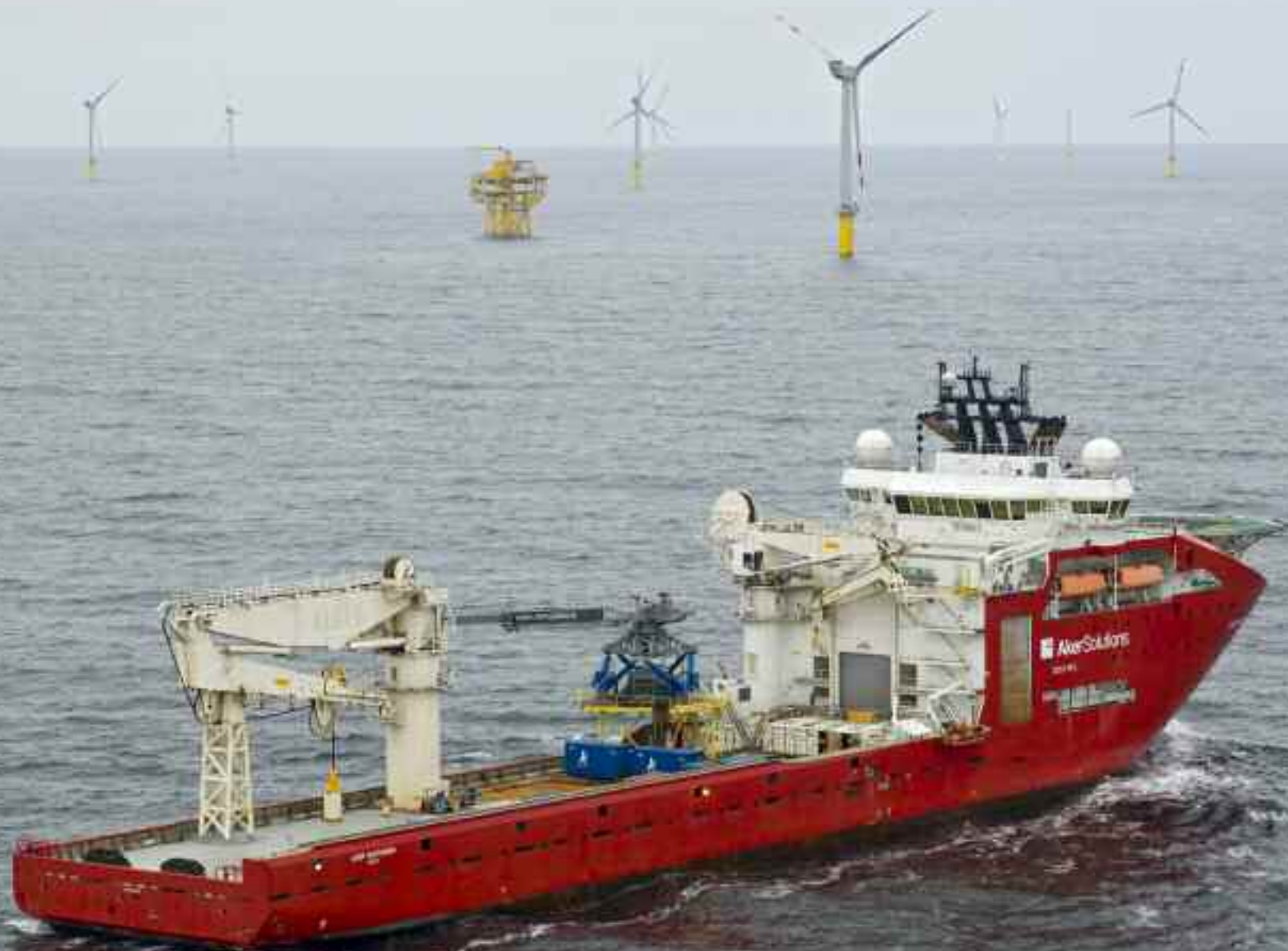
May 15, 2015 – Equipped with two heave compensated cranes and an Ampelmann W2W system the 157 metre long multipurpose construction vessel Aker Wayfarer owned by Aker Solutions from Lysaker in Norway on its way to the Borkum West Offshore Wind Farm.
