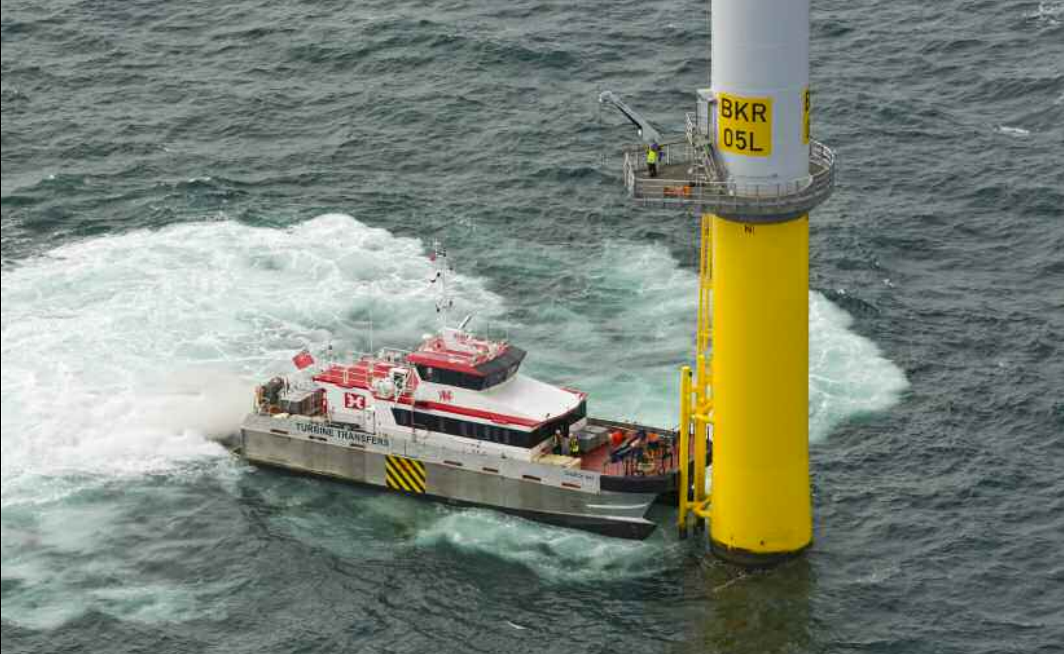
August 5, 2015 – The wind farm support and crew transfer vessel Church Bay of Holyhead Towing's subsidiary Turbine Transfers Limited just transferred personnel on one of the Borkum West wind turbines.
