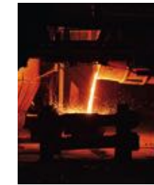
p. 95 Tapping of a steel ladle. Photo Pauline van Lynden.
