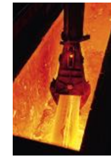
p. 96 Lifting a billet from the reheating furnace, Vallourec Düsseldorf-Reisholz. Photo Pauline van Lynden.
