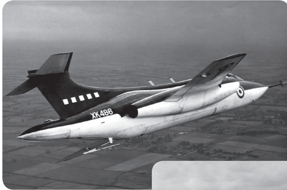
The first NA.39 Buccaneer prototype XK486, with non-folding wings, at an early test flight in 1958. (Blackburn)
