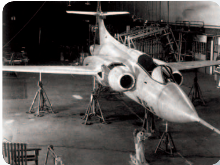
Buccaneer prototype XK486 under construction at Blackburn in the Brough factory. (Blackburn)
