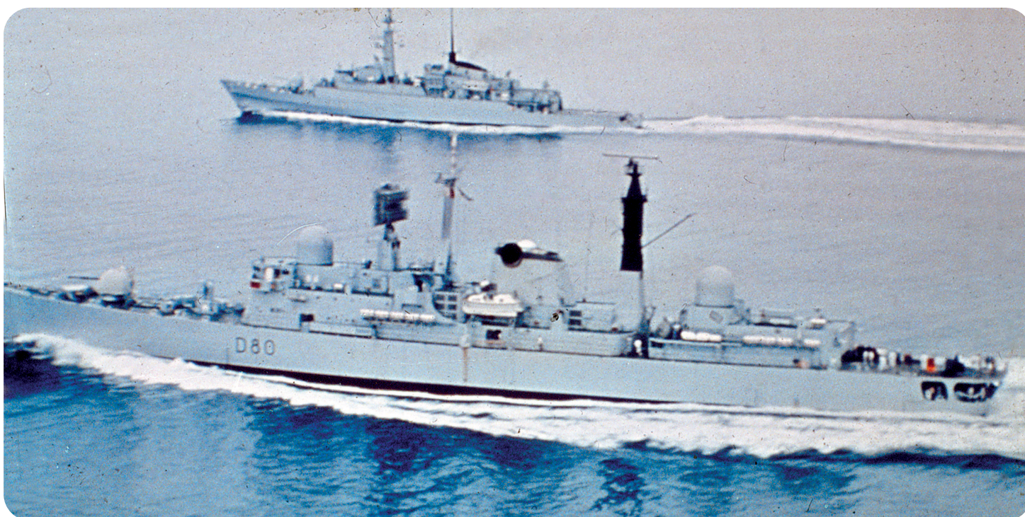
Sheffield on trials. Note the 'Loxton Bends', often called 'Elephant Ears' or 'Mickey Mouse Ears', the prominent exhaust funnels intended to deflect hot exhaust gasses away from radar antennae and flightdeck. They proved unnecessary and were not fitted to the other Type 42s.
