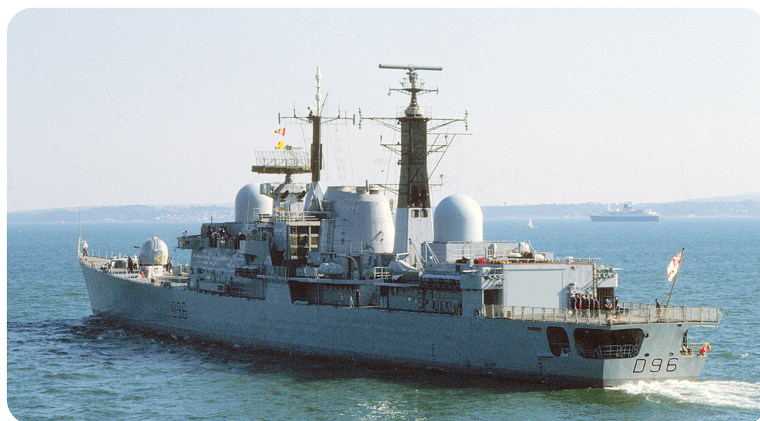
HMS Gloucester was one of the modified of the class. Having a lengthened hull design giving better seakeeping and endurance.
