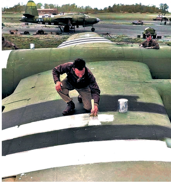
Painting invasion stripes on a B-26 Marauder. A special Operation Memorandum prescribed the size and location of the black and white bands that had to be applied to the U.S. and British airplanes for the invasion of Normandy. In practice, however, the stripes were applied quickly, in a not very exact manner, as this guy does with a large brush. (Life Magazine)
