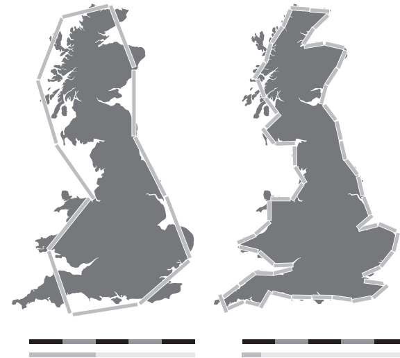
FIGURE 1 The measured length of the coast of Britain is 2400 km (approx.) with a scale unit of 200 km (left side of figure) and 3400 km (approx.) with a scale unit of 50 km (right side of figure) (image retrieved from Van de Sande, 2004).
