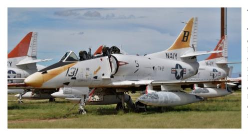
TA-4J 158093 arrived on 18 August 1994 from TW-2. At some point its canopy blew off and it has been dumped under the fuselage. The right fueltank also seems to have received some damage over time, as it is broken in two. It is obvious this 'Scooter' is ready for the scrapman.
