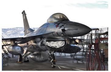
All openings on the upper side of the aircraft are taped. A first layer of black spraylat is applied. This thin plastic coating protects the airframe from dust and water. A second layer of white plastic protects from the sun and reduces the inside temperature by 15 to 20 degrees. This preserves valuable cockpit items.
