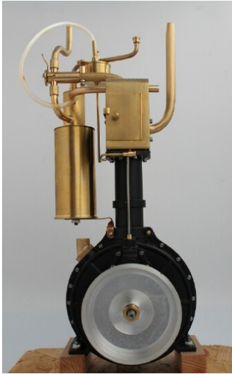
Daimler snellopende benzinemotor
