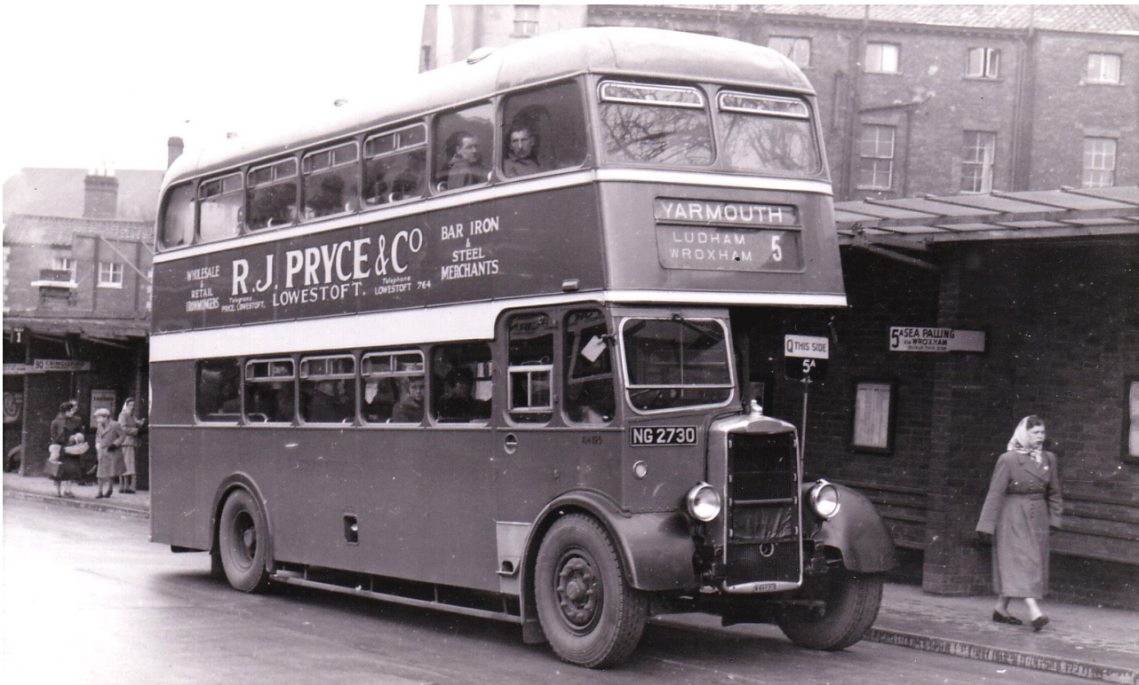
(A195 (NG 2730) a 1932 built Leyland Titan TD2 with ECW 56 seat bodywork, awaiting departure to Yarmouth, via the Broads, from Norwich, Surrey Street bus station, some time during the mid 1950s. This vehicle originally carried an ECOC built body, but received this new post war one in May of 1950, which saw it through until withdrawal some ten years later in 1960, following an amazing 28 years of passenger carrying service!)
