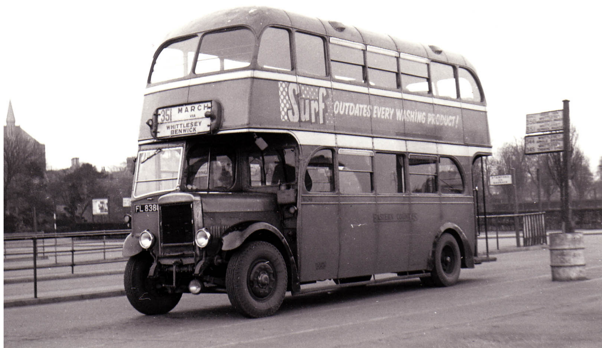
(FL 8380 – a 1930 all Leyland Titan TD1 with 48 seat low-bridge bodywork, seen here after transfer to the new Eastern Counties fleet, awaits departure to March on route 351, via Whittlesey and Benwick from Peterborough's, Bishops Road bus station.)
