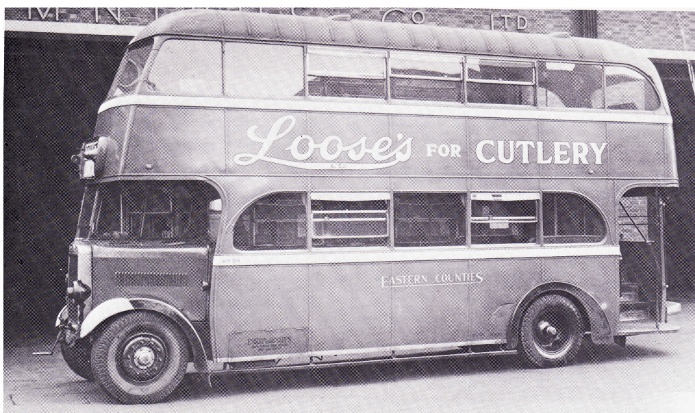
(An unidentified A class Leyland TD2 with 52 seat ECOC bodywork seen here resting outside the Norwich, Surrey Street bus garage c1940. Note the white tipped mudguards and the slit headlamp attachments to comply with wartime regulations. Two similar vehicles were destroyed by enemy action here in 1941.)
