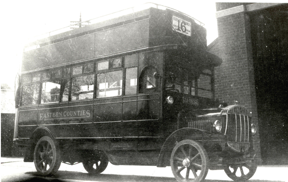
(XA 8692 – a 1920 built Tilling bodied Tilling Stevens TS3 open decked omnibus seating 51 passengers is seen here operating a Bury St Edmunds to Newmarket service in the early days of the Company. This vehicle was transferred to the new Eastern Counties fleet in October of 1931, receiving fleet number PE19.)
