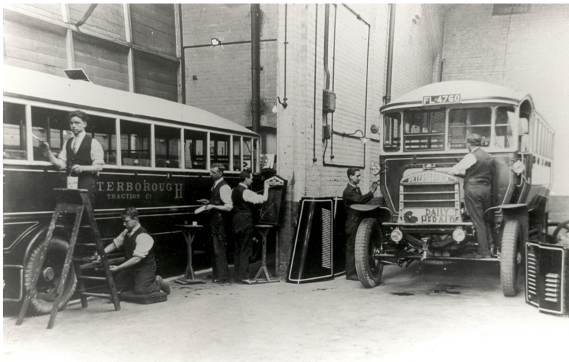
(This fascinating photograph captures FL 4760 – an SOS 'S' type saloon with Ransomes 28 seat bodywork, delivered in 1926, receiving attention from industrious workshop staff in the Peterborough's Lincoln Road paint-shop. This vehicle was transferred to the new Eastern Counties fleet in October of 1931, becoming fleet number S18.)
