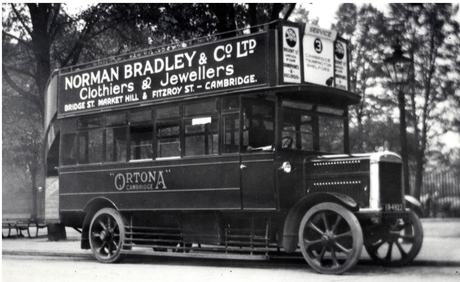
(ER 4922 – a Leyland GH7 omnibus with Dodson 53 seat open decked bodywork was new in 1926 and is seen here in Cambridge awaiting departure on Service 3 to Shelford. This solid tyred vehicle was transferred to the new Eastern Counties fleet in October of 1931 and became their fleet number AA40.)
