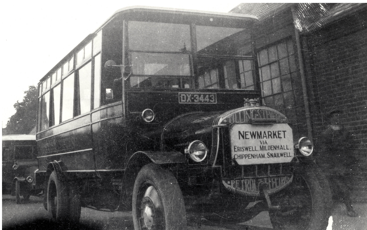
(DX 3443 – A Tilling Stevens Petrol Electric saloon with a 28 seat Tilling body seen outside the Bury St Edmunds garage, awaiting departure to the horse racing capital of Newmarket. This vehicle was one of many considered too old to be transferred to the new Eastern Counties fleet and subsequently disposed of.)
