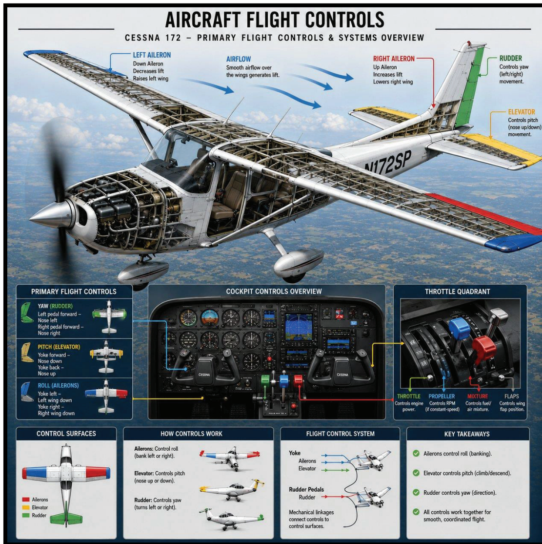
Figure 1.3 — Engine and flight controls. On the left, the throttle quadrant: throttle (power), mixture (fuel/air ratio), and propeller pitch. On the right, the three control surfaces: ailerons (roll), elevator (pitch), and rudder (yaw), plus the propeller providing thrust.
