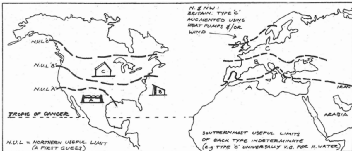
FIGURE 1 Three generic types of solar houses. These types are applicable across most of Europe and North America: A) Skytherm for heating & cooling (classified as a passive system); B) Glazed, heavy south wall for heating and some cooling effect (a passive system, the Trombe Wall belongs to this type); C) Sloping fluid-cooled, heating (an active system). The three types are suitable on areas belonging to particular climatic regions as indicated on the map. The article says that the three types all have something in common with the vernacular architecture of the related climatic region and that they are all economically affordable. They are described as a good starting point with room for improvements and a clear overall principle. (Architectural Design, 1/1976)
