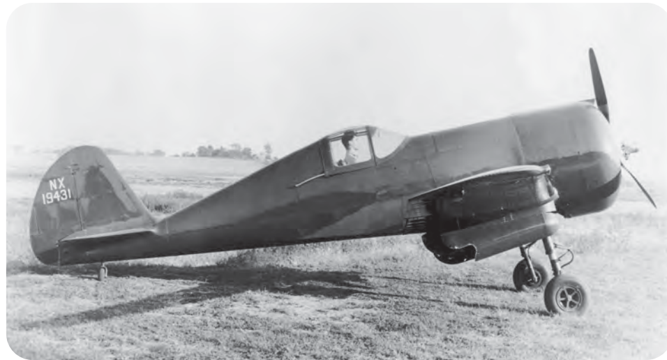
This side view reveals the strongly tapering tail design of the CW-21. The rearwards sliding cockpit hood was supported by an external guide rail. The aiming device, a simple ring sight, was attached to the top of the wind shield. (collection N. Braas)
