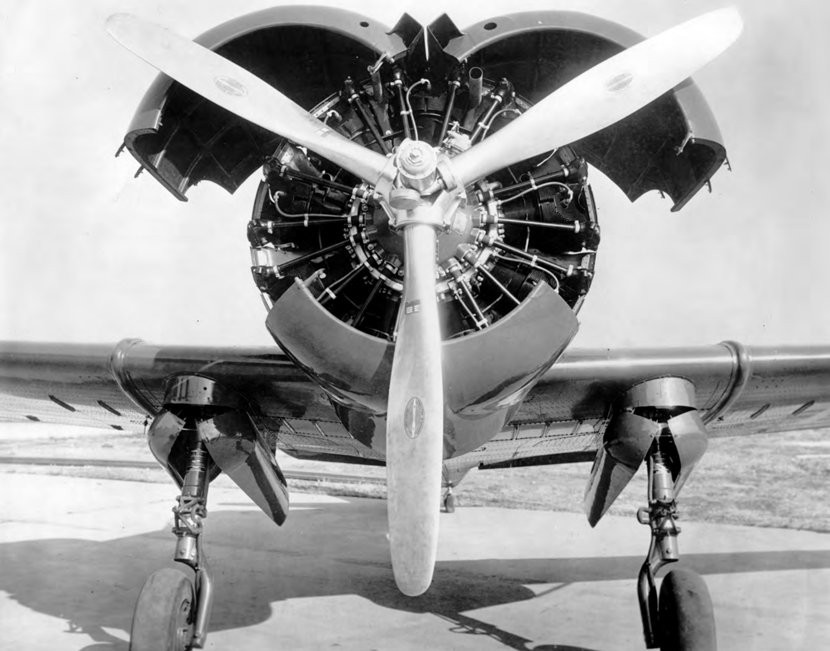
Front view of the Pratt & Whitney R-1820-G5 engine. It was a standard civilian engine but was reliable and power was sufficient. The front view reveals the greater width of the starboard blast tube, suggesting that a .50 machinegun may have been fitted. (collection E. Hoogschagen)
