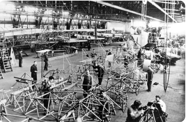
Production of different Fokker types, with four C.XIws in various stages of assembly. In front is the first series D.XXI intended for Finland. Behind those a Fokker T.IVA fuselage is seen.
