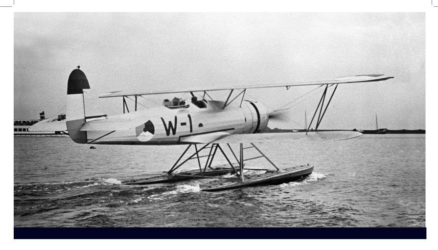
The W-1 prototype is ready for a test flight. During testing, some edges of the fuselage panelling were taped over as a precautionary measure. The prototype featured a Scarff ring in the rear cockpit. (Collection: N. Braas)
