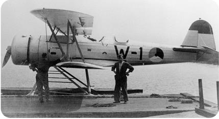
The prototype before a flight to Germany. Its civil registry is not yet applied, but the gun ring is removed, and the rear cockpit coaming is modified.
