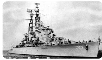
In August 1976 *De Zeven Provinciën* was renamed *Aguirre*. RIM-2 Terrier SAM removed, replaced by a hangar with large flight deck for three ASH-3D Sea King helicopters. Decommissioned 1999.
