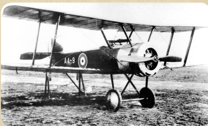
Further development of the Tabloid resulted in the Pup; a very docile and maneuverable fighter. This one with registration A4-9 served in the Australian air force after the end of the war.
