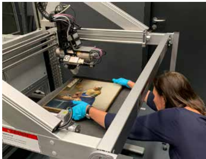
FIG. 9 Rijksmuseum paintings research scientist Annelies van Loon placing The Milkmaid (cat. 8) under the MA-XRF scanner
