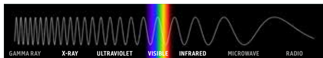
FIG. 1 Electromagnetic spectrum illustrating the range of radiation types applied in the examination of paintings
