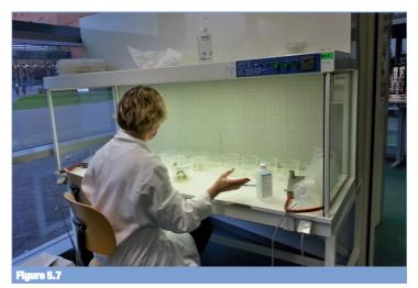
A horizontal laminar flow cabinet blows air into your face; it is only suitable for work with harmless materials and microorganisms.
