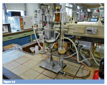
Glassware and tubing of setups are particularly subject to wear. Connections may loosen over time and start to leak.
