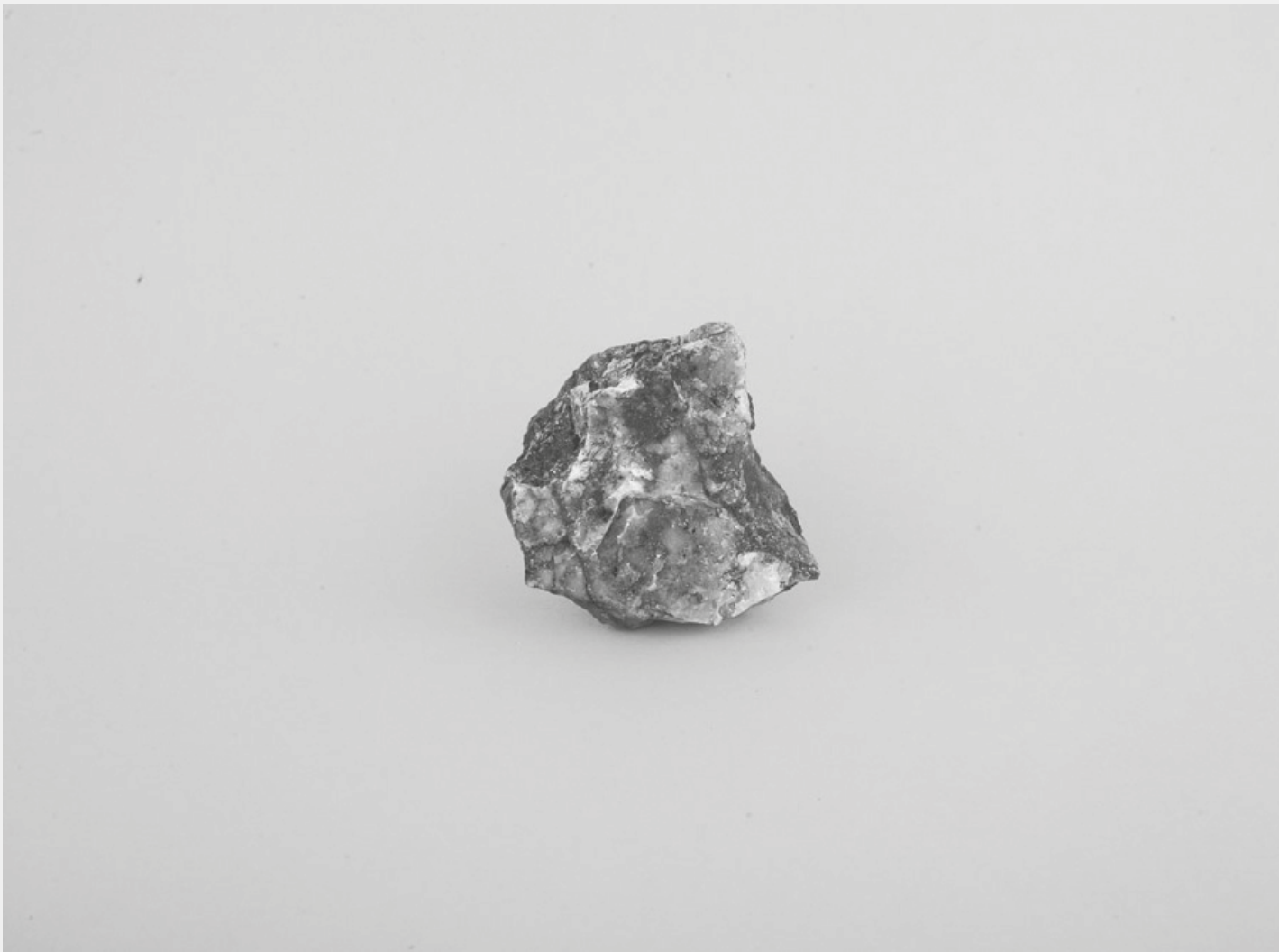
fig a Arsenic Rock. Zuckenhut mine, Gasen. Photo: Simon Brugner. ~ This 7-cm-in-diameter rock sample was collected in a historical arsenic mine. It consists mostly of quartz and arsenopyrite, an iron arsenic sulfide. These stones were hand-sorted, crushed, and roasted. The toxic smoke, arsenic trioxide, often simply referred to as “arsenic,” was passed through horizontal chambers where it would condense into solid form.
